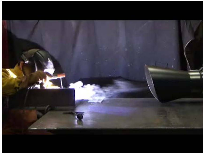
Figure 5: Hood 2 diameters from arc with hood ON THE TABLE Welder: 2.195 \mu\text{g}/\text{m}^3
