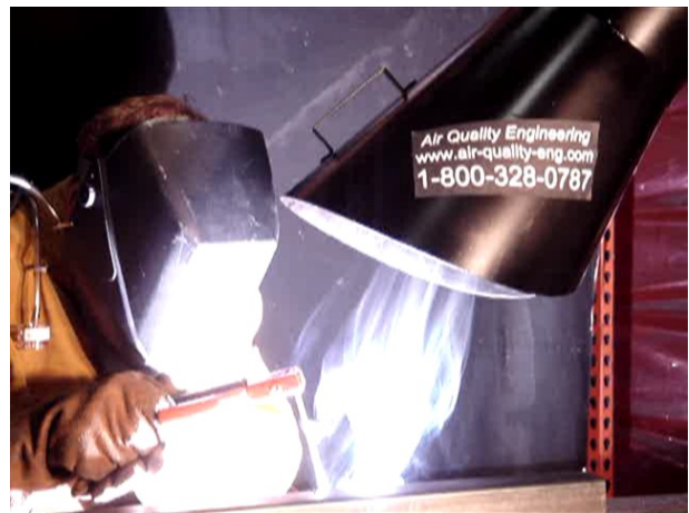
Figure 2: Hood 1 diameter from the arc: Welder: 2.075 µg/m 3
