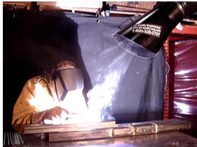
Figure 4: Hood 2 diameters from the arc: Welder: 13.722 \mu\text{g}/\text{m}^3
