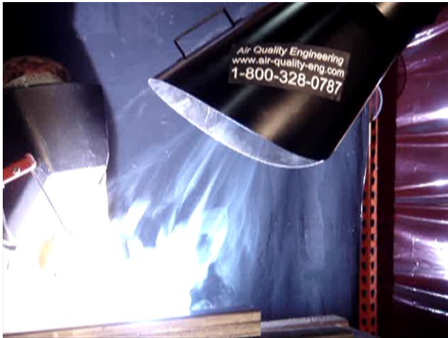
Figure 3: Hood 1½ diameters from the arc: Welder: 2.222 \mu\text{g}/\text{m}^3
